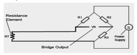
The simplest resistance thermometer configuration uses two wires. The wiring arrangement utilises a wheatstone bridge, it comprises of 4 equal value resistors. When all 4 resistances are the same, the bridge is said to be 'in-balance', resulting in no output through Vb. However, when one of the arms of the bridge changes in resistance, the bridge becomes unbalanced, and an output is the detected in Vb, proportional to the out of balance of the circuit.
