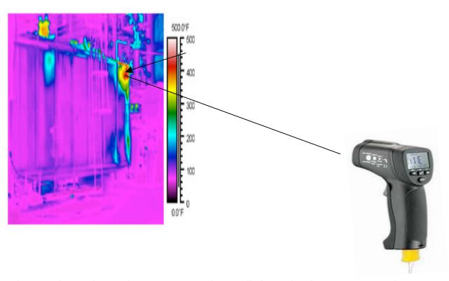
Alternatively, a radiation thermometer, may be installed into the plant structure, as this next
