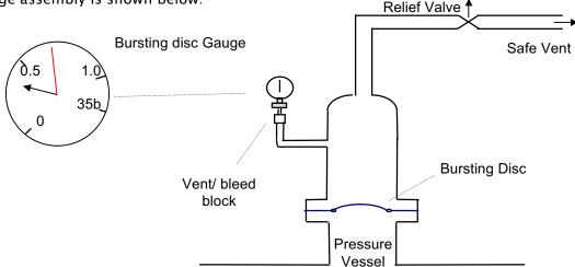
The bursting disc is so designed to rupture when the pressure beneath it exceeds a predetermined safe working limit, prior to this occurring a small pressure may build up, in the
