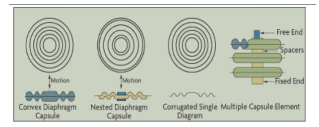
In all cases, the operation of these devices relies on the small amount of flex in the metal, or its 'elasticity'. Eventually though, after constant use, and chemical attack, this elasticity reduces, and the measuring elements require replacement.
