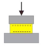
Piezo-electric crystals are man-made or naturally occurring crystals that produce a charge output when they are compressed, flexed or subjected to shear forces. The word piezo is a corruption of the Greek word for squeeze. In a piezo-electric transducer a mass is attached to a piezo-electric crystal which is in turn mounted to the case of the transducer. When
