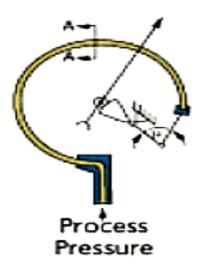
the tube moves outward pulling the quadrant via the connecting linkage, thus in turn turning the pointer via the rack and pinion. The movement of the pointer being linear to the pressure increase. A hairspring is attached to the pointer and gears to remove slackness.
