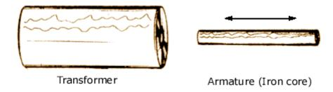
The LVDT is a variable-reluctance device, where a primary center coil establishes a magnetic flux that is coupled through a mobile armature to a symmetrically-wound secondary coil on either side of the primary.
