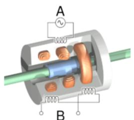
LVDTs are commonly used for position feedback in servomechanisms, and for automated measurement in machine tools and many other industrial and scientific applications.
