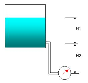
The overall pressure acting on the transmitter is:H1 + H2, where H2 is the static head pressure and H1 is the actual level in the tank. This error (effect of H2) may be eliminated by suppressing the zero.
