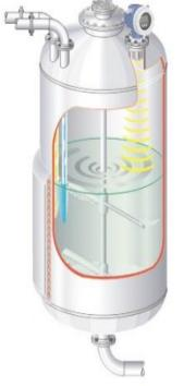
The Ultrasonic Non-Contact Transmitter electronics sends an electrical signal to the transducer sensor crystal, which causes the crystal to vibrate and emit an ultrasonic pulse. The sound pulse is directed toward the liquid surface where
