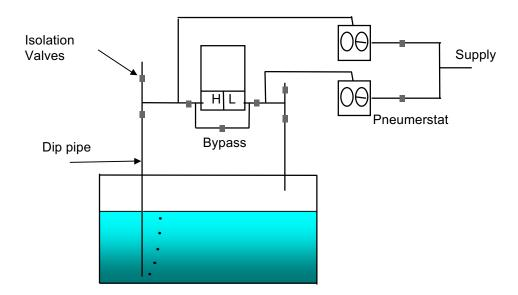
From the previous diagram, when the tank is empty the same pressure acts on both sides of the transmitter therefore creating a zero reading, when the level rises only the high pressure side is affected. If the pressure inside the vessel changes the effect is automatically compensated for. Care should be exercised when operating the isolation valves as the vessel may be under pressure.
