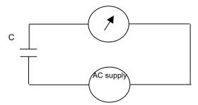
Capacitance level detectors are also referred to as radio frequency (RF) or admittance level sensors. Admittance is a measure of the conductivity in an ac circuit, and is the reciprocal of impedance. Admittance and impedance in an ac circuit are similar to conductance and resistance in a direct current (dc) circuit. AC supply is required, (1) to avoid problems associated with polarization
