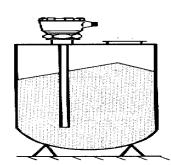
The use of these systems can be similar to the conductive system, however a popular use is to measure liquid interface levels, as the final diagram shows:-
