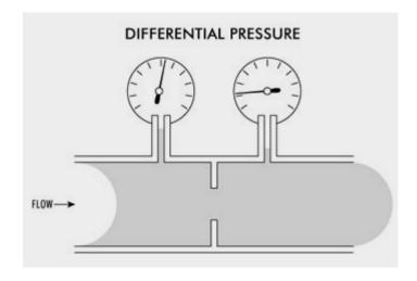
Because of the nonlinear relationship between flow and differential pressure, the accuracy of flow measurement in the lower portion of the flow range can be degraded.
