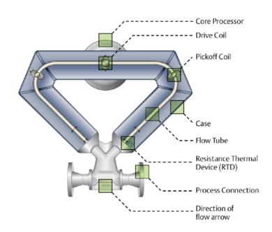
as it flows down the tube (due to coriolis force), and the vibration along the tube becomes non-uniform, resulting in the tube twisting slightly. The amount of twist, causes a phase difference in vibration between the inlet to the tube and the outlet, the amount of which is proportional to the mass flow rate of fluid passing through the tube(s).
