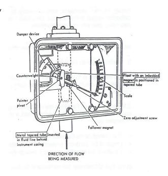
Both the glass and magnetic versions must be periodically removed, cleaned and inspected whilst accuracy can only be checked by passing through a known flowrate in a given time period.
