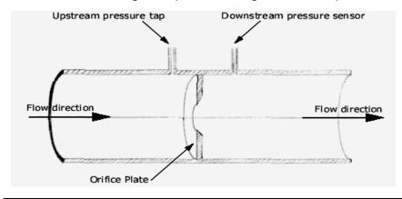
causes an increase in velocity and decrease in pressure. The pressure difference before and after the orifice plate is measured, is used to calculate the flow velocity.
