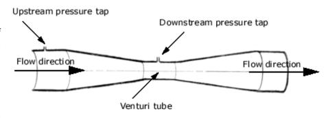
changes in cross section area cause changes in velocity and pressure of the flowing fluid. Bernoulli's equations can be used to relate these changing quantities into flow rate.
